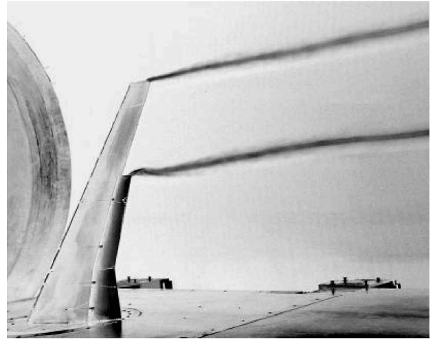
Fig. 7 Smoke visualization of the wing tip and flap edge vortex for \delta_i = \delta_o = 20 deg at \alpha = 8 deg.
