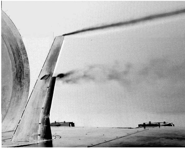
Fig. 17 Smoke visualization of the wing tip and flap edge vortex for \delta_i = \delta_o = 20 deg at \alpha = 9.53 deg with fin at \varepsilon_F = 20 deg.
